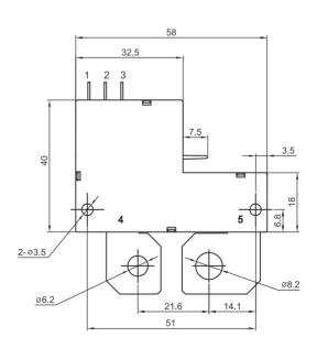
Note: No tolerance marked. If dimension  $\leq$ 1mm, the tolerance is  $\pm$ 0.2mm; if dimension 1-5mm, the tolerance is  $\pm$ 0.3mm; if dimension  $\geq$ 5mm, the tolerance is  $\pm$ 0.5mm.
